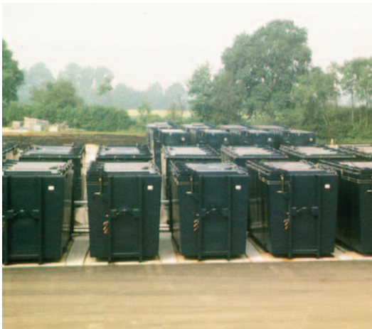
Figure 4.1b: Container composting with controlled aeration (Photo by Ina Körner, courtesy Hamburg University of Technology).
