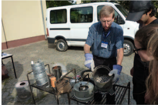
Figure 2.10: Top-lit up-draft (TLUD) micro gasifier stove practical course by Paul Anderson during the 1st international biochar Summer School in 2012 (Potsdam, Germany).
